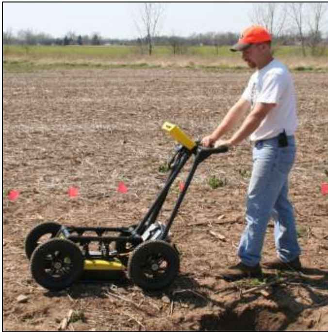
Figure 83: Ground-penetrating radar system used during the survey.
