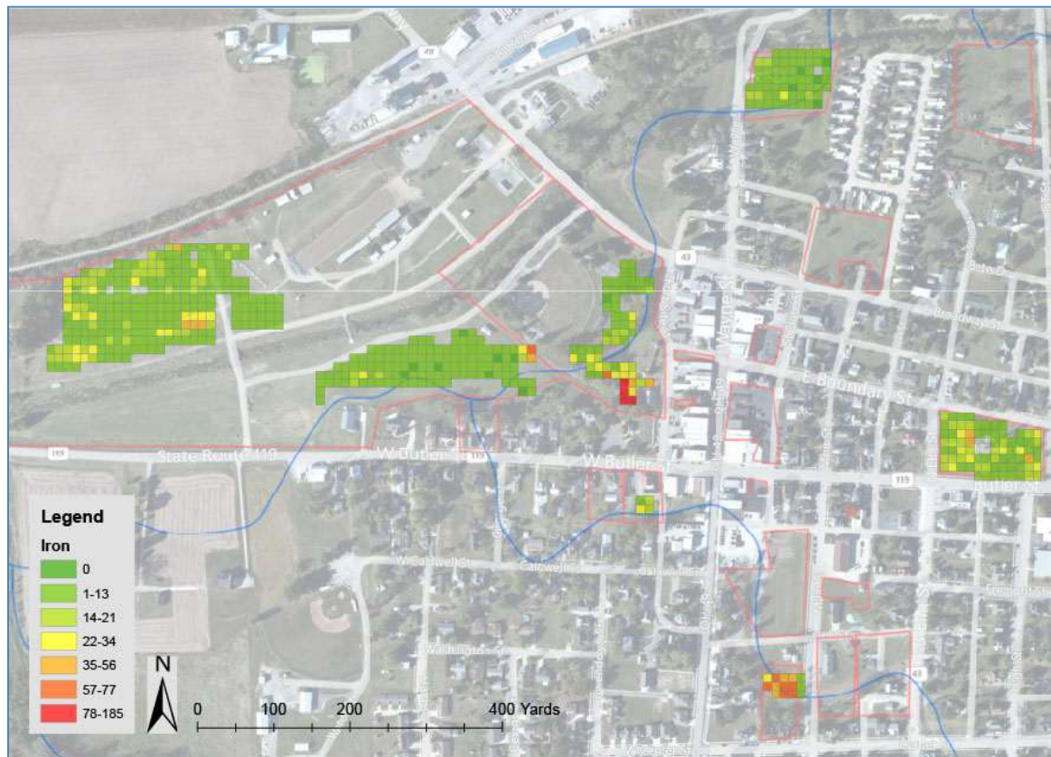
Figure 38: Areas of metal detector surveys with red showing highest levels of metal concentration.
